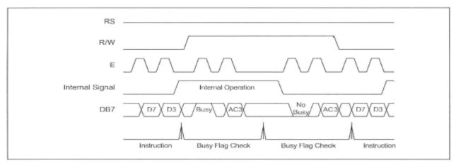
Example of 4-bit Bus Mode Timing Sequence
