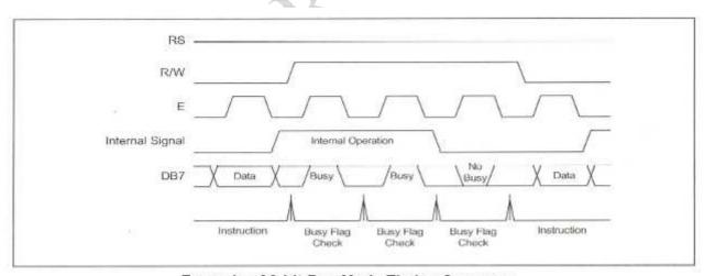
Example of 8-bit Bus Mode Timing Sequence
